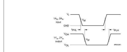
$V_M = 1.5 \text{ V at } V_{CC} \ge 2.7 \text{ V};$
